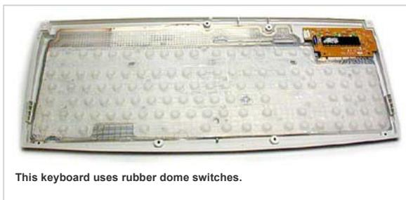
This keyboard uses rubber dome switches.
