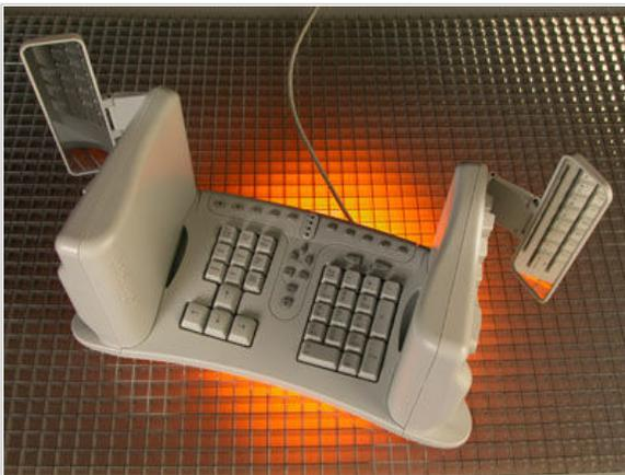
The SafeType keyboard places the two halves of the keyboard perpendicular to the desk surface.
